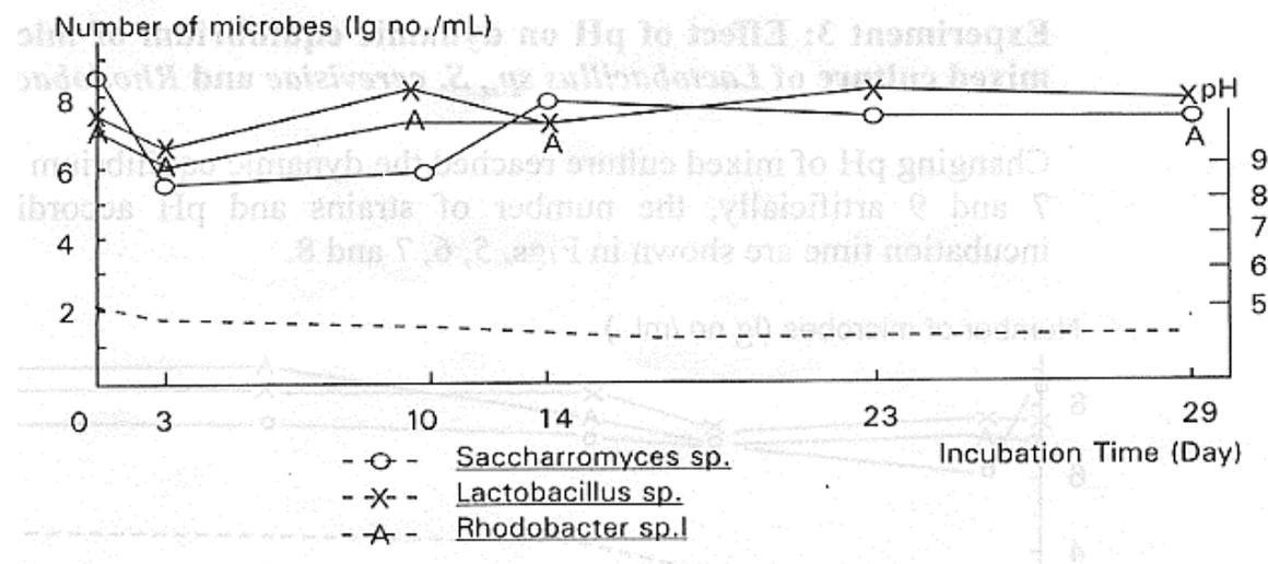
**Fig. 7. Controlled pH of Dynamic Equilibrium of Mixed Culture to pH 7, Change in Microflora According to the Incubation Time.**
