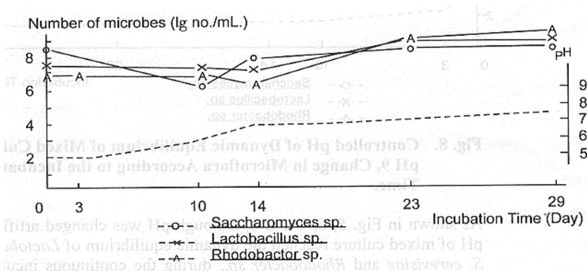
**Fig. 6. Controlled pH of Dynamic Equilibrium of Mixed Culture to pH 5, Change in Microflora According to the Incubation Time.**
