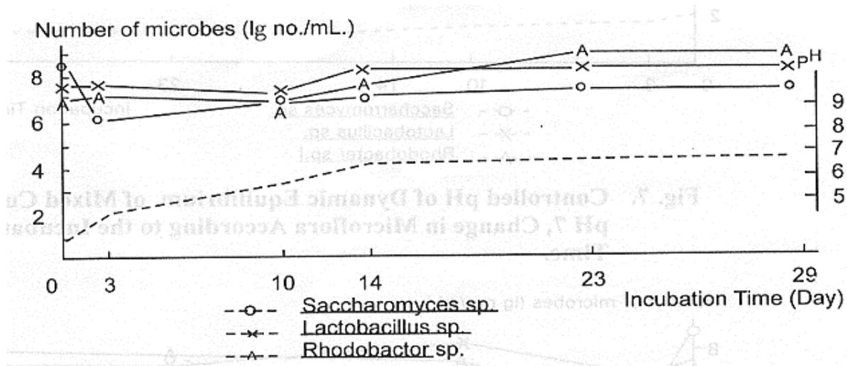
**Fig. 5. Change in Microflora According to Incubation Time when pH of the Dynamic Equilibrium of Mixed Culture was Controlled to pH 3.**
