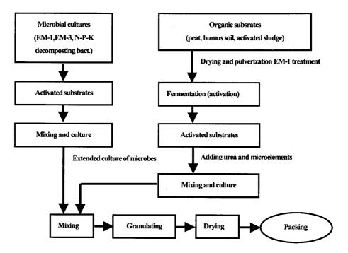
Figure 2. Manufacturing Process of Multi-ingredient Compost
