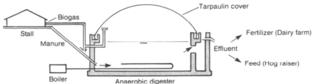
**Figure 1. Schematic Diagram of Flexible Dome Type Digester.**
