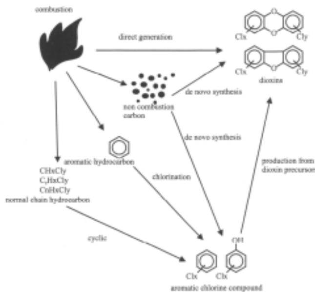
**Fig 2. Main Sources of Dioxin Production through Combustion in Trash Incinerators**
