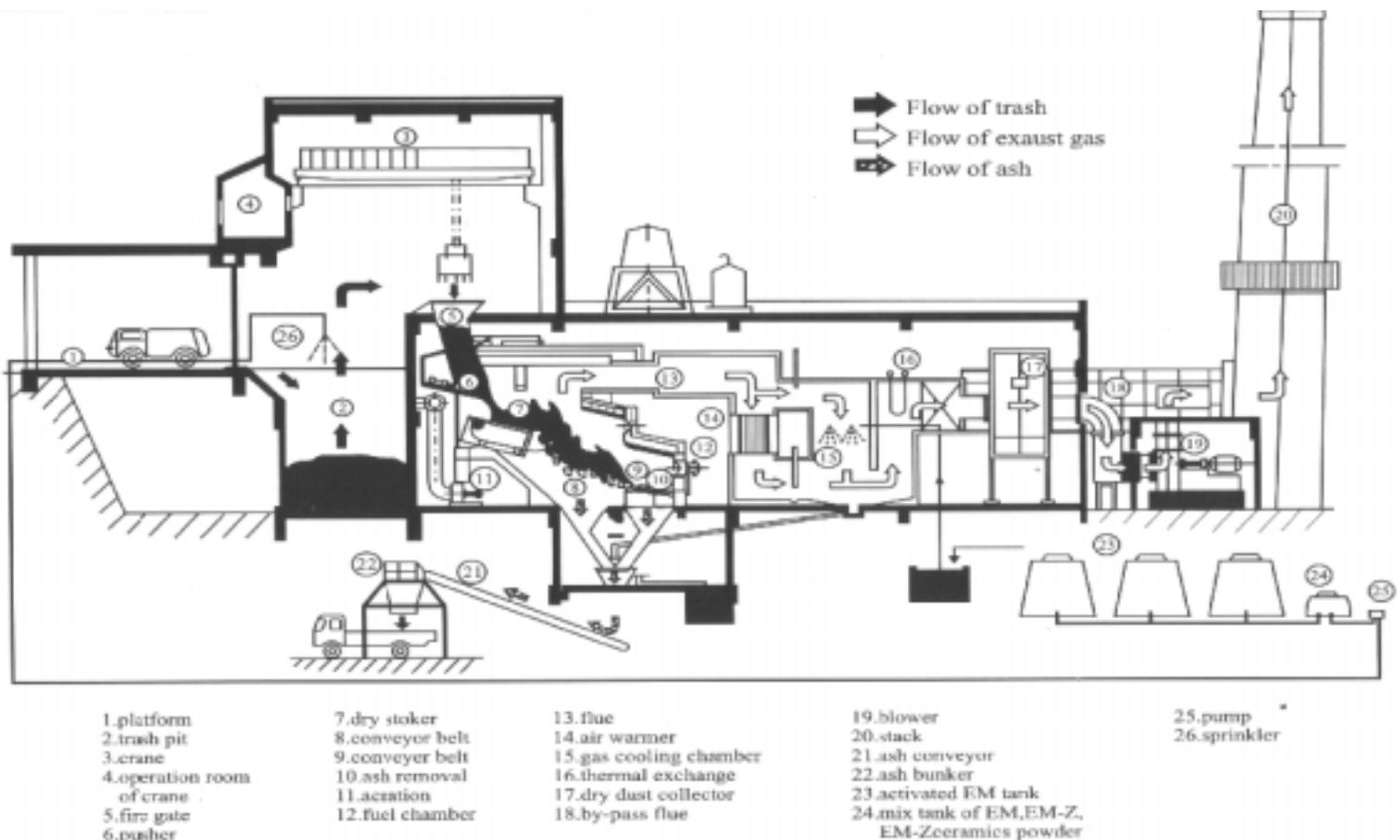
**Fig 3. Flow Diagram of the Gushikawa Municipal Incinerator**
